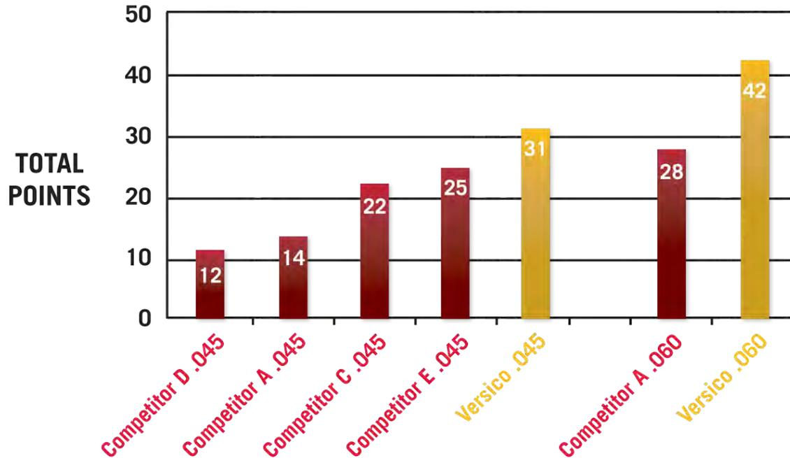
After compiling all of the test data, a ranking system was applied to each of the TPO membranes. Each test was given the same weight in terms of importance. For each of the tests, the sample that performed the worst was given a score of 1, and the sample that performed the best was given a score of 7. Therefore this table reflects the cumulative score of all the tests.
