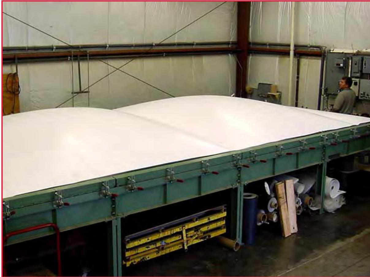
Simulated Wind Uplift Test - The stronger the seam, the greater the uplift resistance.
