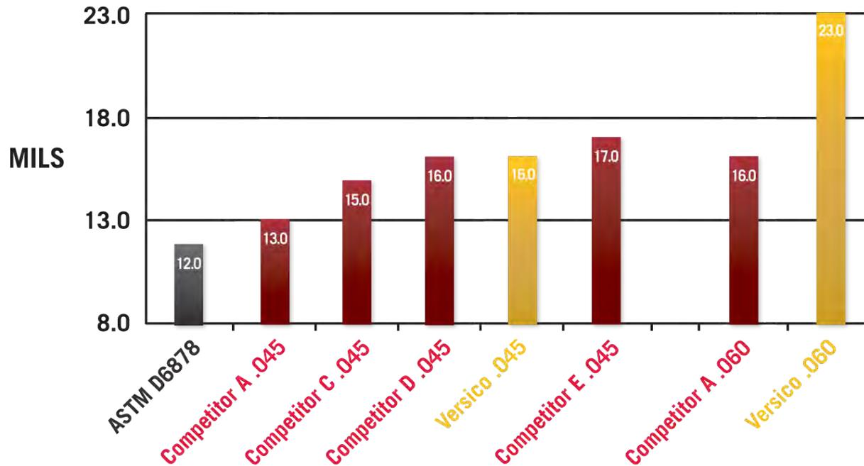
While it's important to have a thick sheet, which is measured in the "Thickness Overall" test, "Thickness Over Scrim" measures the top-ply of the TPO membrane. TPO consists of a top-ply, scrim in the middle and a bottom ply. The top-ply is the front line of defense against the elements and the usable life of the membrane is compromised when the scrim is exposed. Thickness over scrim is a critical measurement when evaluating the potential longevity of a TPO roofing system.
